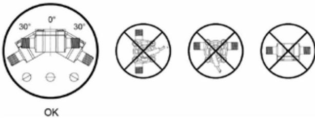
**IMPORTANT:** Flow sensor requires horizontal mounting. Maximum 30 degree tilt
